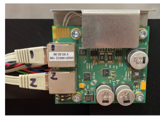
Stepper Control PCB Main
